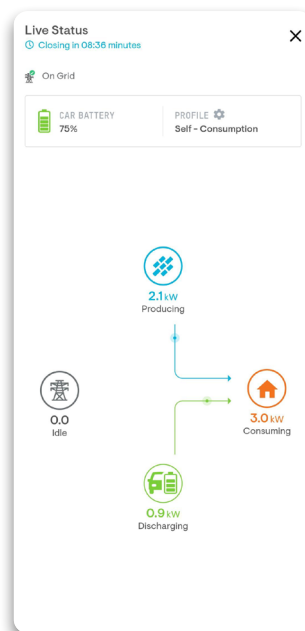
Figure 9: Net-zero import from grid. Managing home loads through solar and EV battery
