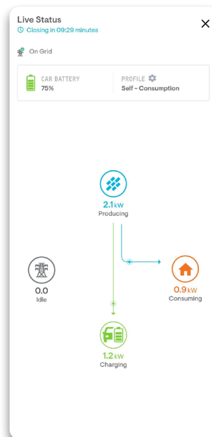
Figure 8: EV battery charging only from Solar
